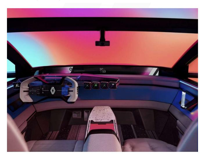
The LED-based coloured lights Appear throughout the interior for added on-board comfort. A reading light has been added to the front passenger door for greater reading comfort. Each head rest also features a LED light for added comfort and lighting.
