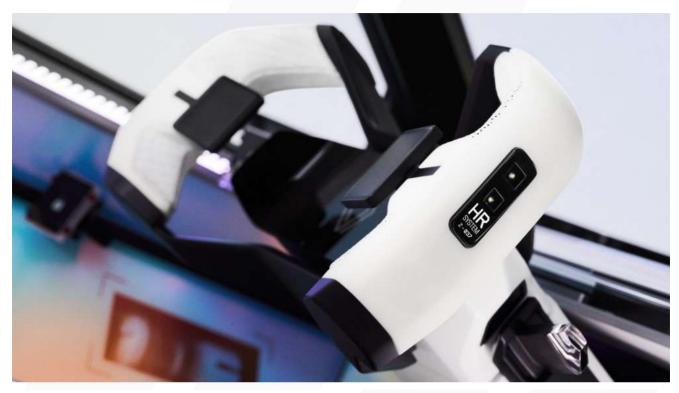
To further drivers, the vehicle comes fitted with an array of health monitoring systems. A heart rate sensor placed in the steering wheel and a camera serve to detect signs of driver fatigue or idleness. Should a problem arise, warning signals are sent to the driver and passengers.
