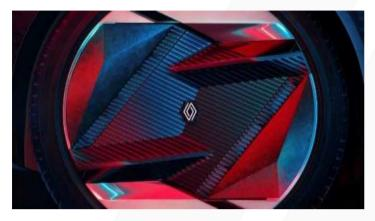
Fitted with large 21-inch wheels, the rims on the Renault Scenic Vision are equipped with flaps for enhanced aerodynamic performance, and therefore greater efficiency. When the car is in motion (≥ 10km/h), the flaps close to improve their aerodynamics; as soon as the car slows down and its speed drops below 10km/h, the flaps open for better cooling as the heat generated by the brakes can escape more readily. A specific mechanism has been added to
