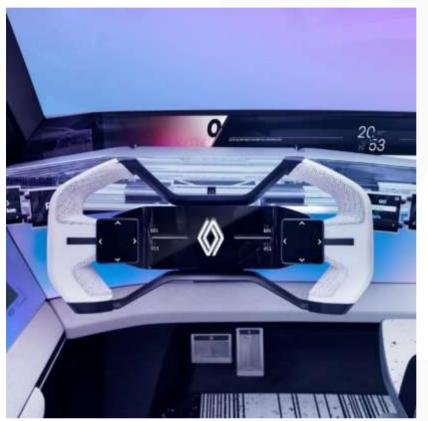
The Renault Scenic Vision comes equipped with a very large screen located where the windshield meets the dashboard, as close as to the horizon line as possible. The goal is to give the driver the best possible view. Its position maximizes ergonomics and safety by preventing the driver from taking their eyes off the road as they look for information which is displayed in two distinct areas: one for the driver, one for the passenger.
