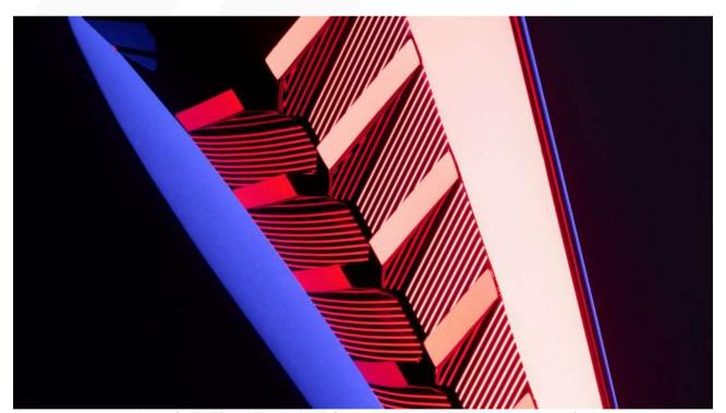
The rear quarter-window is framed by a clear outline of lights: thin lines light up to show tha car's charge level, and to also indicate when the car is unlocked. The light is built into a colourless aluminium panel, and serves to underscore the new silhouette's strong sense of character.
